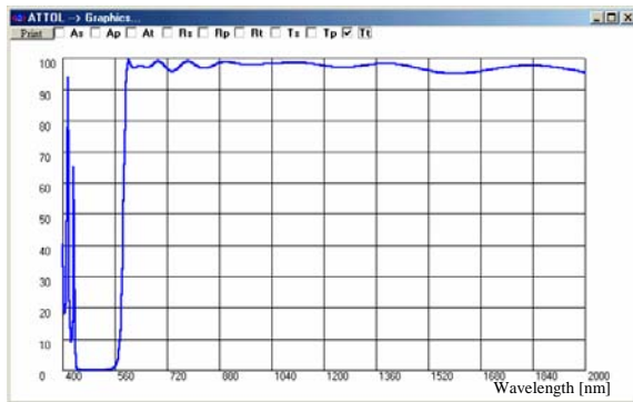
Fig. 6-b. The theoretical curve of a spectral transmission for an optimized interferential filter for 600 - 2000 nm spectral domain, having the formula (19).
